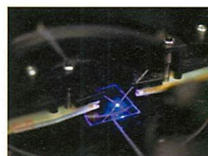
First InGaN-LED chip in Yamaguchi Univ.
